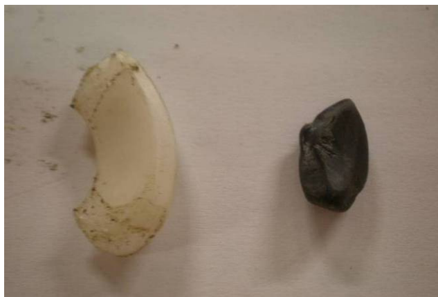
Figure 2 – Close-up of debris found in a check valve
