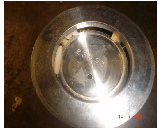
Figure 1 – Teflon debris trapped in check valve
